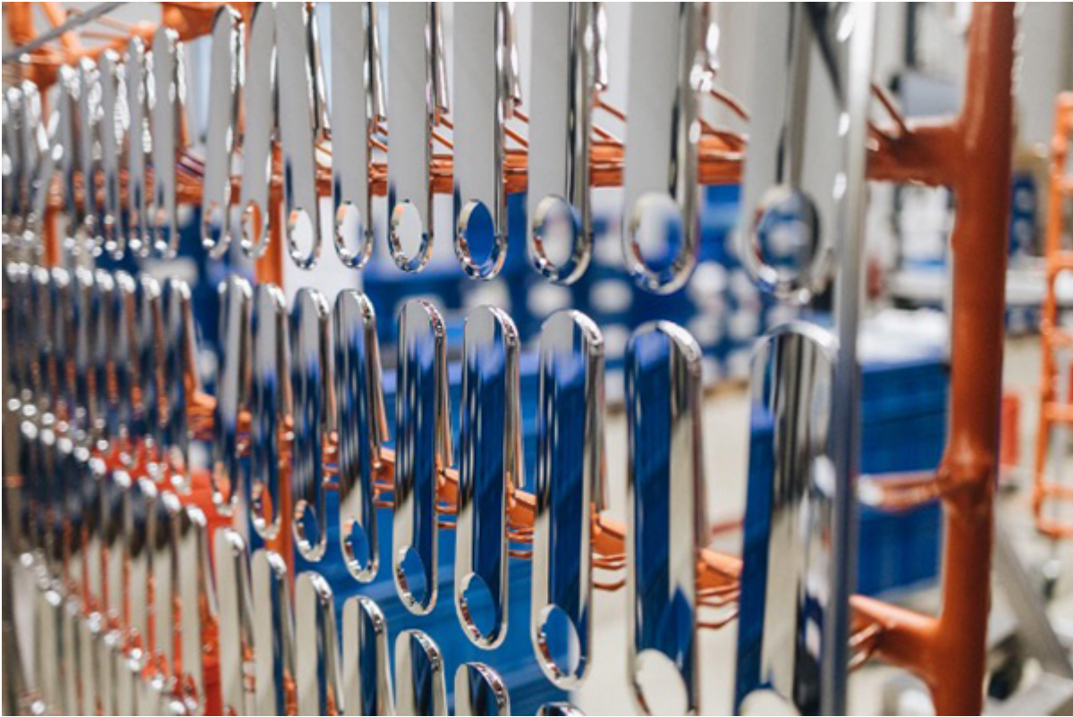
Faucet handles being plated for a high gloss aesthetic and protection against corrosion and blemishes.
